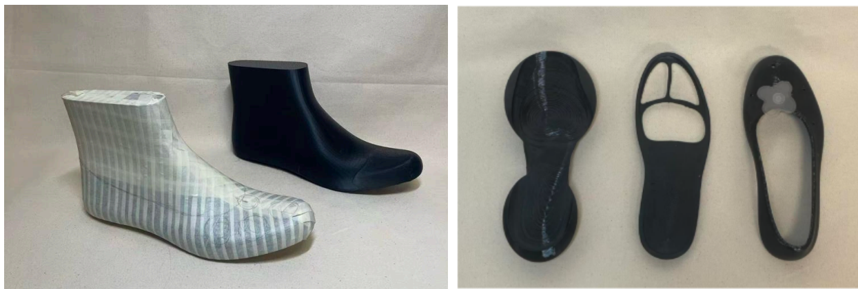
[Figure 5.30: 3D printed shoe last; traditional pattern-making on last to establish base form and unit positions]
