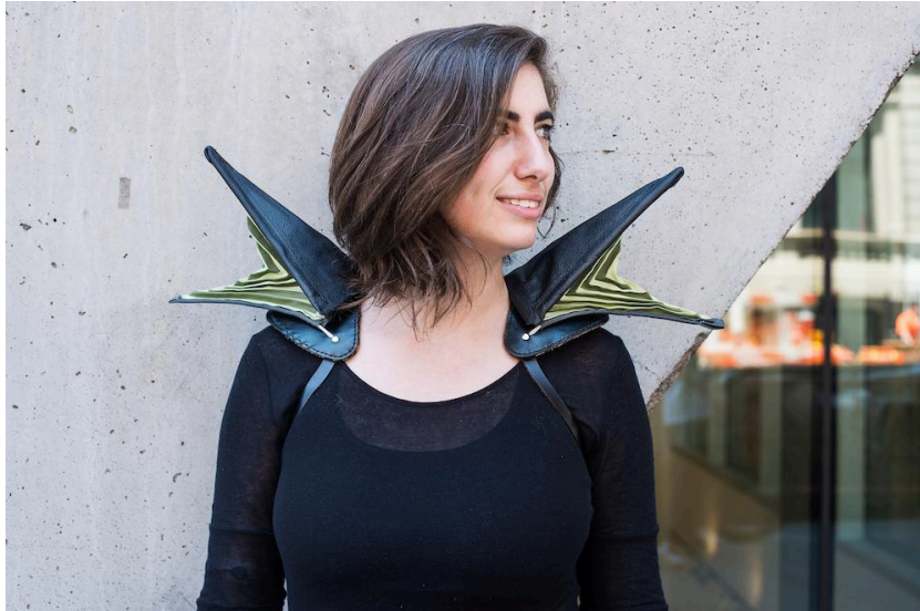
[ Figure 3.4. Monarch V2, a shoulder-mounted wearable with EMG-driven pleated textile forms that amplify body presence. From "Monarch: Self-Expression Through Wearable Kinetic Textiles," by K. Hartman et al., 2015, Proceedings of TEI '15. Copyright 2015 by ACM.]
