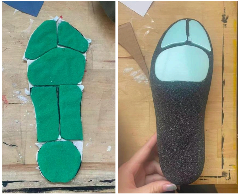
[Figure 5.29: Sensor zone comparison: initial 6-zone design vs. final 3-zone layout on insole, with forefoot trigger zones]
