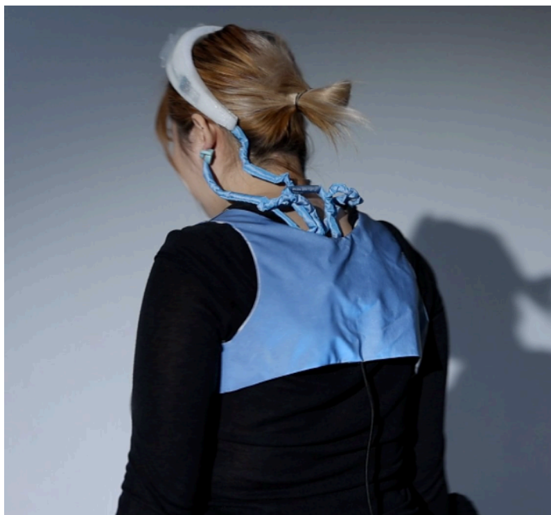
[Figure 5.5. Full headwear system worn from the rear, showing how the headband, ear-clip sensor, and component-housing vest connect across the body.]
