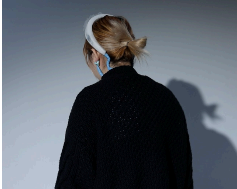
[Figure 5.4. Rear view of the headband, showing the pulse sensor cable routed from the ear-clip down behind the neck.]
