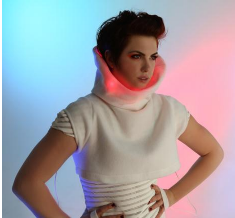
[Figure 3.7. GER Mood Sweater, translating galvanic skin response into LED color changes in a tall collar. From "GER Mood Sweater," by K. Neidlinger / Sensoree, 2013 ( https://sensoree.com ). Copyright 2013 by Sensoree.]
