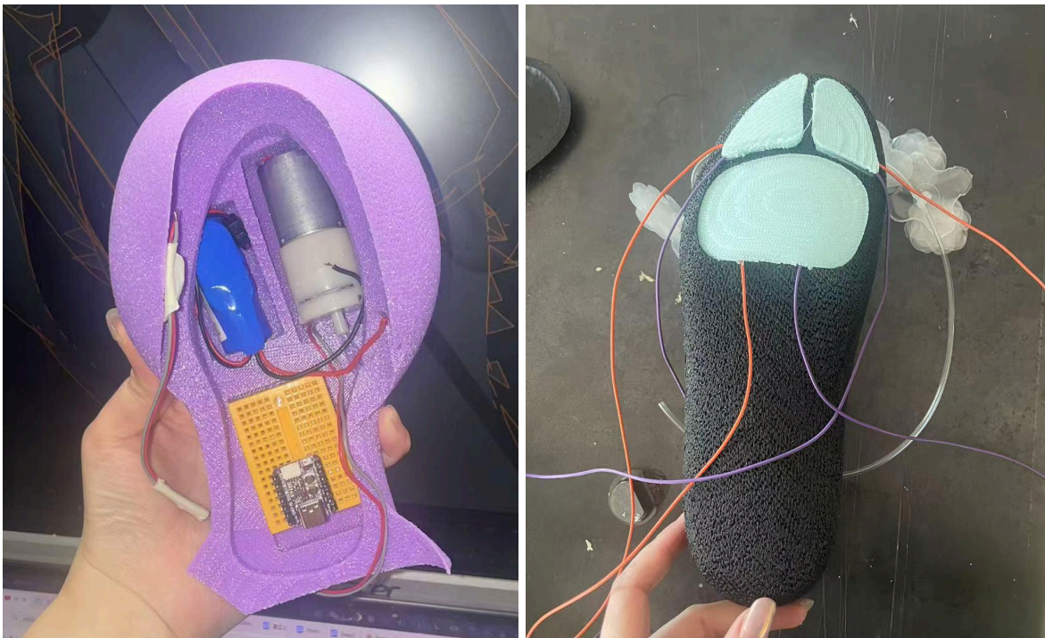
[Figure 5.32: Cutaway of final sole showing internal component layout: QT Py, battery, pump, wiring, and charging port position and modular sensors placed in liner]
