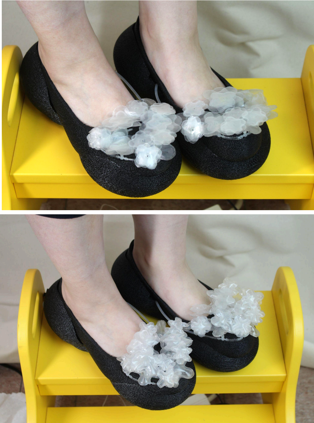
[Figure 5.33: Top view of footwear showing unit placement on dorsal surface; deflated (relaxed) vs. inflated states(nervous/awkward)]
