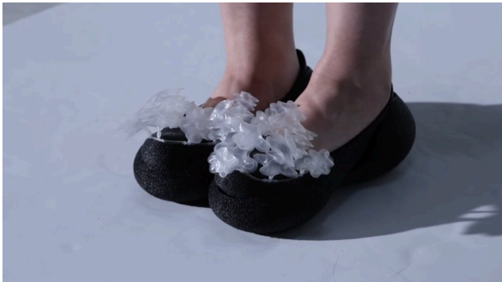
[Figure 5.3. Plantar pressure-responsive footwear worn, with inflation units expanded across the upper following toe-gripping activation.]
