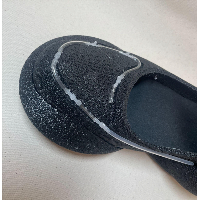
[Figure 5.34: Cross-section of upper showing embedded tubing channels routing from units down to sole]
