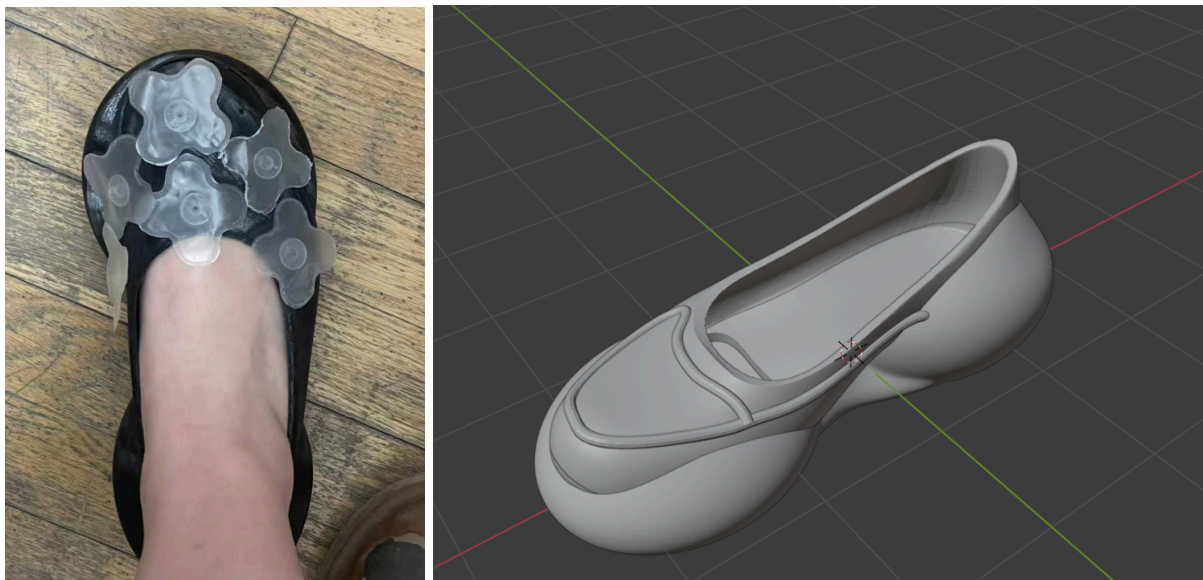
[Figure 5.31: Design sketch with unit positions marked in prototype 1; 3D model showing integrated tubing channels; printed prototype being tested for fit]
