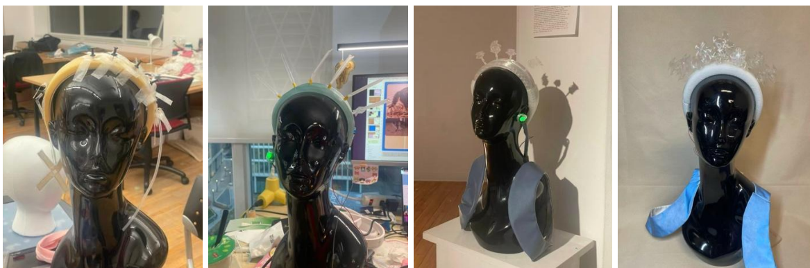
[Figure 5.22: Headband evolution: (a) V1 modified craft store headband with externally attached components, (b) V2-V4 3D printed headband with internal cavities for pump housing]
