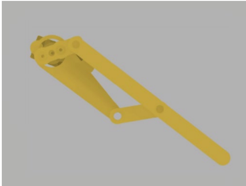
Figure 20 Initial AWORM Leg Design (3D Render)
