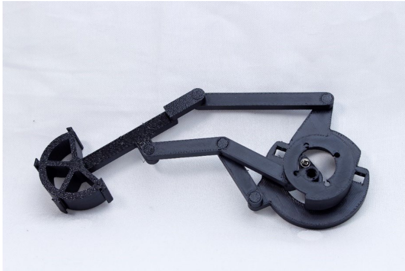
Figure 25 AWORM 5-Bar Linkage Leg
