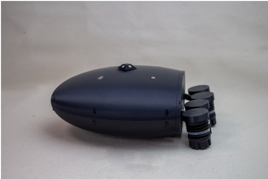
Figure 21 AWORM with a Later Leg Design with Rubber Foot
