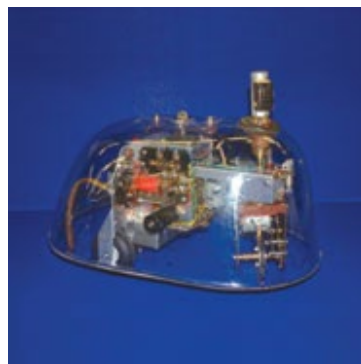
Figure 18 Modern replica of Grey Walter's tortoise, with perspex shell
