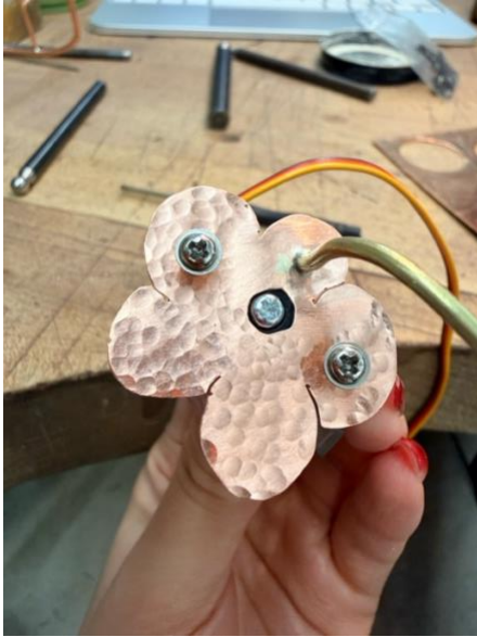
Figure 20. Hammered copper plate used as a connection and reinforcement element for the wing structure.
