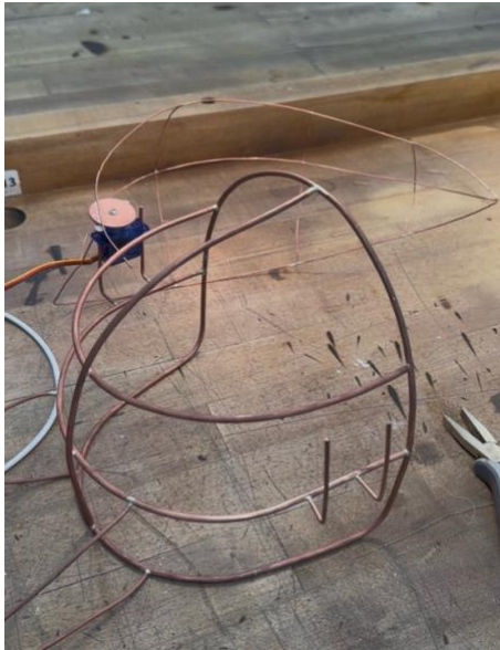
Figure 18. Copper wire structure of Folding wings
