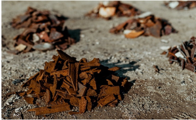
Figure 29. fragmented radiators and break routers laid out as charges for the furnace. Felion studios February 2026. Photo by Rob and Samantha Dutcher.
