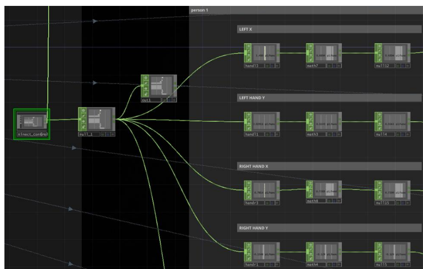
Figure 20. Hand-axis extraction and routing in TouchDesigner. Kinect hand position data separated into four channels (Left X, Left Y, Right X, Right Y), then routed through processing and mapping nodes to prepare values for OSC/MIDI output.
