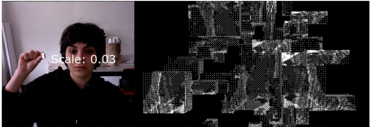
Figure 12. (left) MediaPipe hand-tracking test in TouchDesigner showing thumb-index pinch distance (“Scale”) used as a continuous control signal. (right) Generative block field under high-noise condition produced by a closed pinch gesture (low thumb-index distance)
