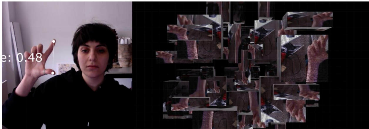
Figure 12. (left) MediaPipe hand-tracking test in TouchDesigner showing thumb-index pinch distance (“Scale”) used as a continuous control signal. (right) Generative block field under high-noise condition produced by a closed pinch gesture (low thumb-index distance)
