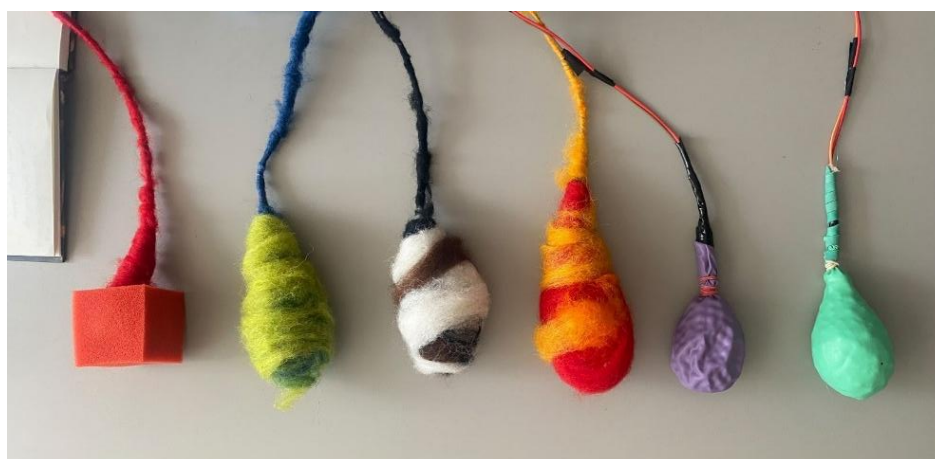
Figure 7. Early material prototypes for pressure interaction (FSR embedded in silicone, wool, foam, balloon with jellybeans, fidget balls, and fabric-wrapped forms).
