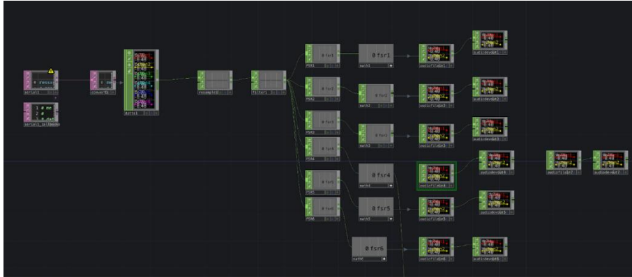
Figure 11. TouchDesigner signal conditioning and channel separation: serial data converted to CHOP, smoothed with Resample and Filter CHOPs, split into FSR1–FSR6 using Select CHOP, then scaled/clamped with Math CHOP for audio volume control.
