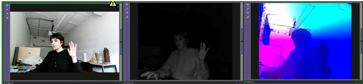
Figure 17. TouchDesigner Kinect TOP set to (in left to right order) Color, Infrared and point cloud mode. Screenshot by author. The Kinect TOP provides selectable image streams (including Infrared and Depth) from Kinect v2 for use in low-light interactive setups.
