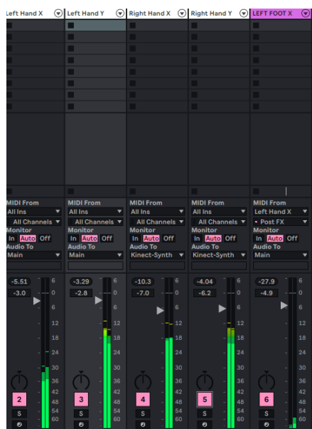
Figure 22. Ableton Live session view with movement-driven MIDI tracks. MIDI tracks mapped to hand axes (Left Hand X/Y, Right Hand X/Y) receiving data from TouchDesigner and driving distinct sonic layers; meters show active modulation during gesture input.
