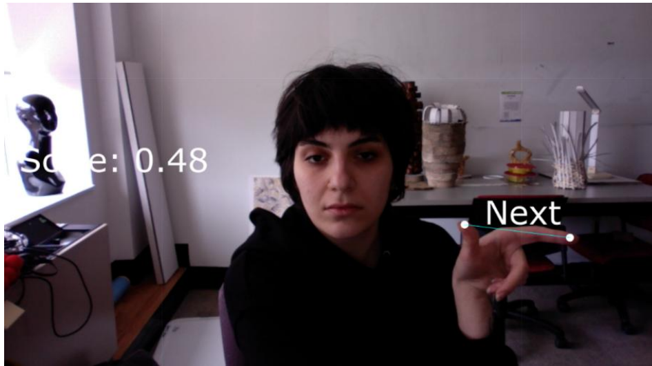
Figure 14. Gesture-trigger test: rotating/turning the index finger to the right triggers a “Next” state change, re-seeding the positions of the moving blocks and activating a brick-like sound cue as confirmation.
