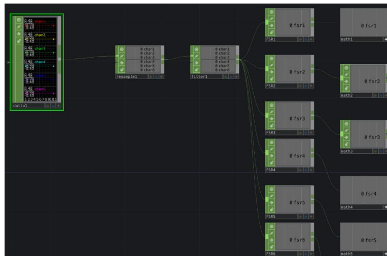
Figure 10. TouchDesigner prototype network for receiving six-channel pressure data via Serial DAT, converting it into CHOP signals, and routing each sensor channel into an audio feedback chain.
