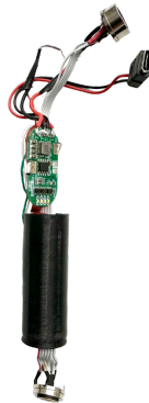
Figure 20: The unsuccessful prototype of the Battery Bank module, highlighting the wiring and exposed circuitry that failed and needed to be disassembled out of the carbon fiber shaft.
