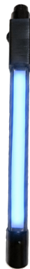
Figure 22: The Light Bar module, integrating a vertical RGB LED strip to improve user visibility and environmental illumination in low-light conditions.
