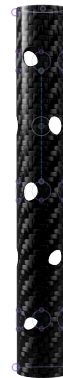
(c) 3D render of the modified carbon fiber shaft displaying the final machined hole pattern.
