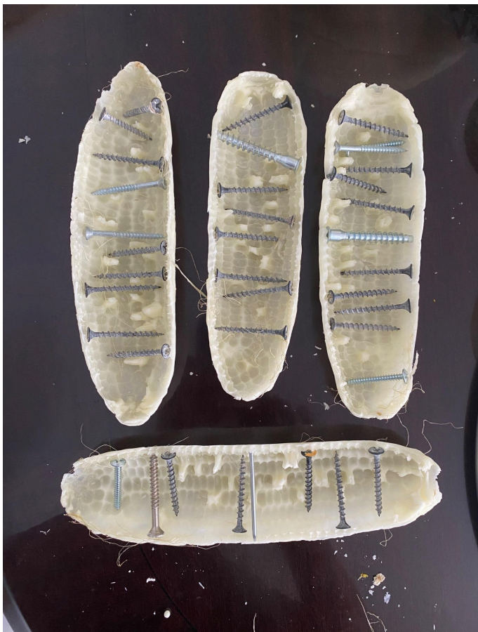
Figure 17. Mold made of cornstarch. Photo by Hugo Bernilla, 2025.
