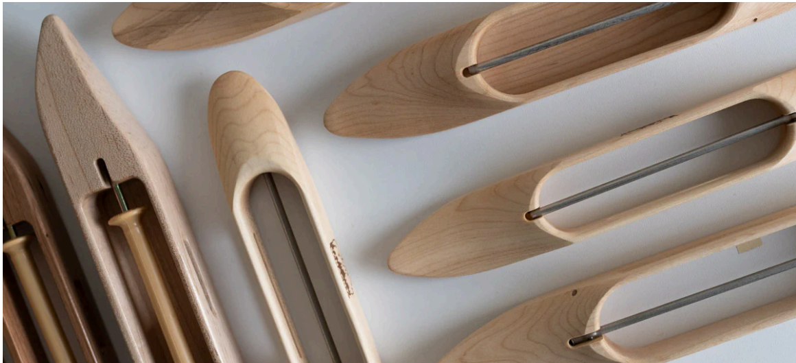
Figure 17. Examples of wooden boat shuttles, showing the pointed profile and hollow bobbin-holding body typical of this shuttle type. Note. From “All About Shuttles,” by Gather Textiles (n.d.), Gather Textiles .
