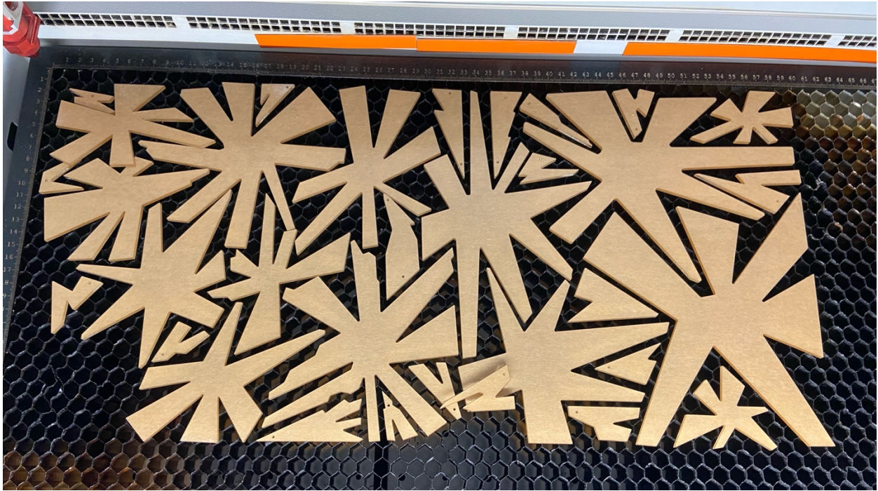
Fig. 22: Laser-cut clear acrylic star forms before peeling off the protective layer.
