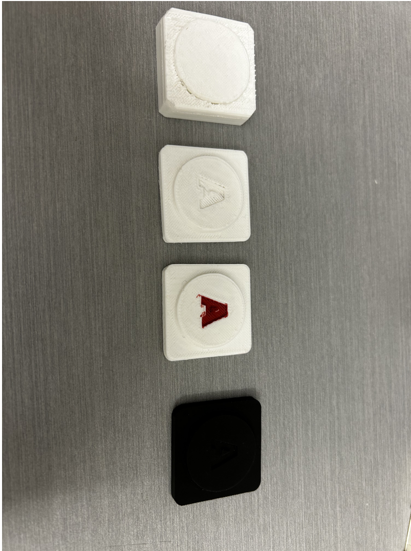
Figure 4.1: Keycap prototype evolution showing iterative refinement: (1) initial white prototype with circular indent, (2) arrow symbol variant for directional keys, (3) two-color inlay experiment with red arrow, and (4) final black keycap design using black resin material.
