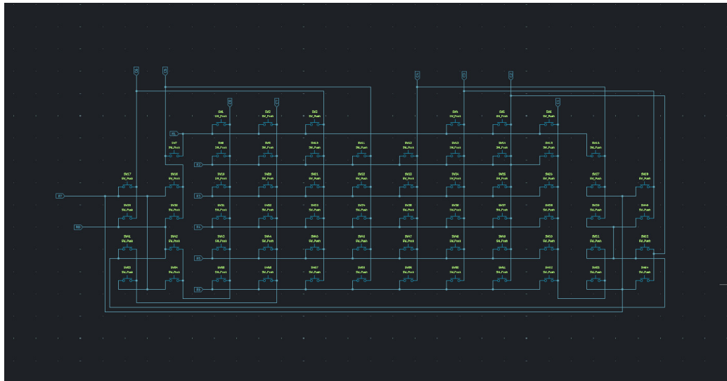
Figure 5.7: Final keyboard schematic design in KiCad. Unlike the initial version, this schematic reflects the correct matrix logic with the 8 \times 8 column-row connections visible as the complex routing pattern connecting all 64 switches.
