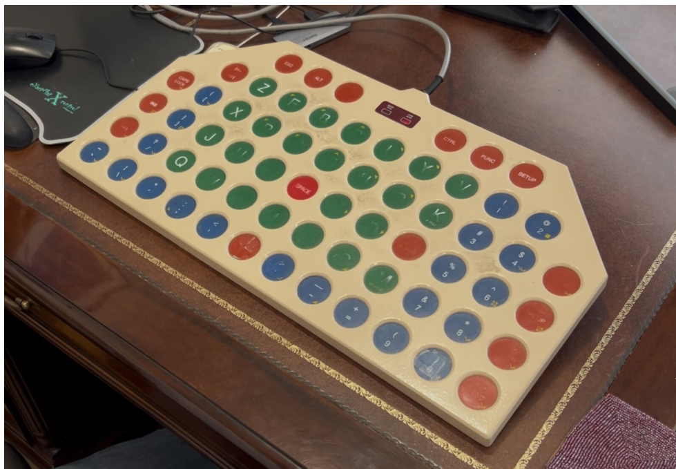
Figure 1.1: The original King Keyboard, a custom accessible keyboard developed with Jutta Treviranus's help that Rick has used for decades. The color-coded circular keycaps and distinctive hexagonal form factor accommodate Rick's motor patterns.
