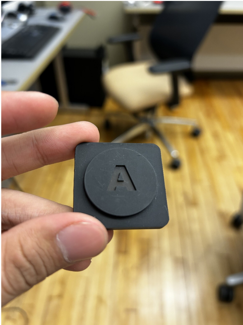
Figure 5.9: Resin keycap prototype printed at OCAD University’s rapid prototyping lab. Rick responded positively to its sturdiness, confirming the material choice would withstand his forceful keystrokes.
