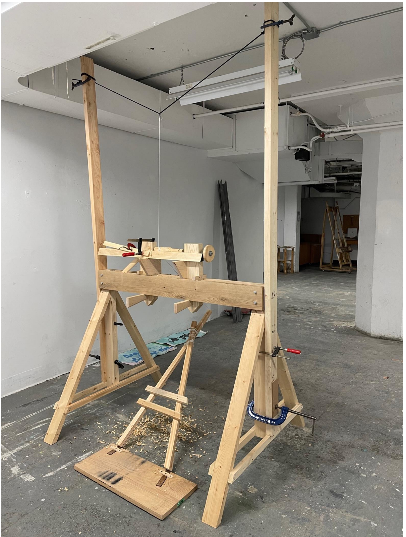
Figure 2. Pole lathe in the basement of OCAD University. The uprights have yet to be bolted onto the A-frames. Oak, ash and SPF, bungy cord, nylon cord, leather. August 2022
