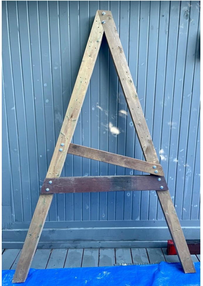
Figures 11-14. Making a riving frame. Used for controlled splitting of logs before they are shaped further on the shaving horse. Pressure treated 2 x 4-inch SPF and reclaimed wood. June 2024.
