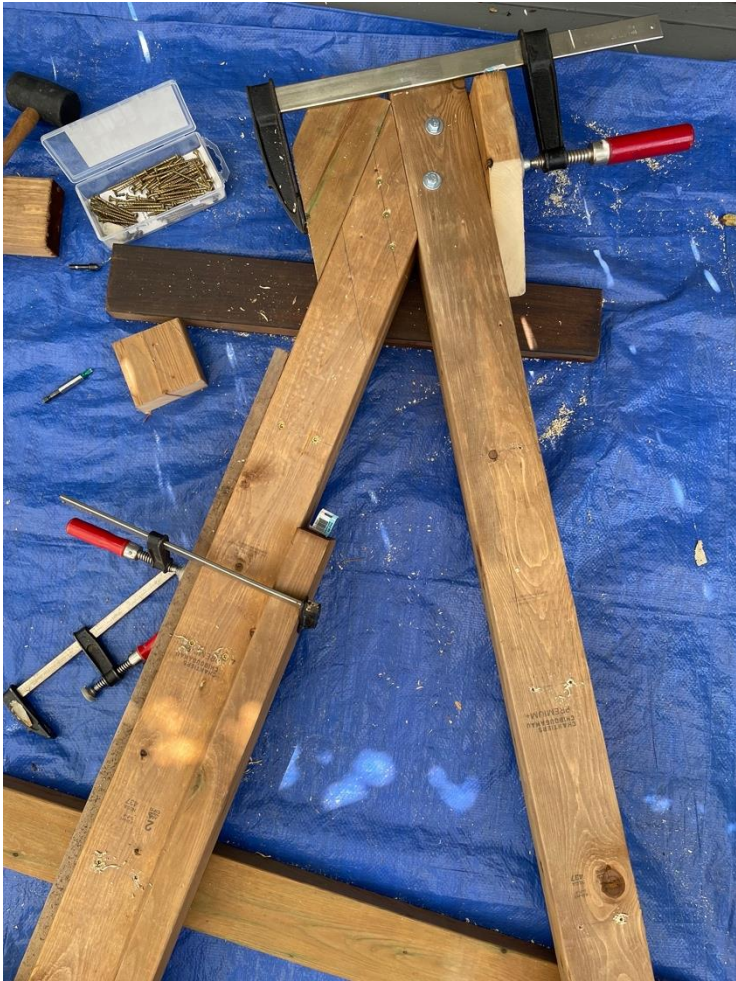
Figures 11-14. Making a riving frame. Used for controlled splitting of logs before they are shaped further on the shaving horse. Pressure treated 2 x 4-inch SPF and reclaimed wood. June 2024.
