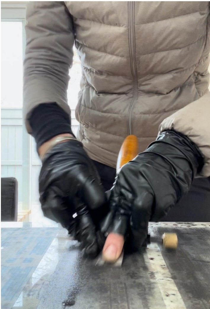
Figures 17-18. Left: Sharpening a 1½ inch chisel on aluminum oxide abrasive film stuck to a granite slab. Right: Evidence of previous uneven sharpening shown on the top right corner of the blade. This must be completely removed to produce one bevel.
