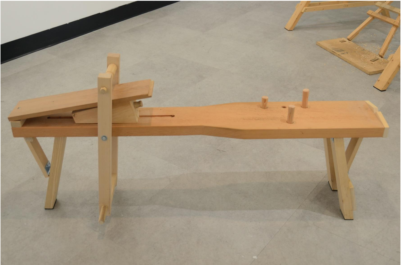
Figure A8. Shaving horse. The pegs shown on the right can be used to grip lengths of wood to be sawn or shaped. Douglas fir, maple, ash, cherry. April 2022.
