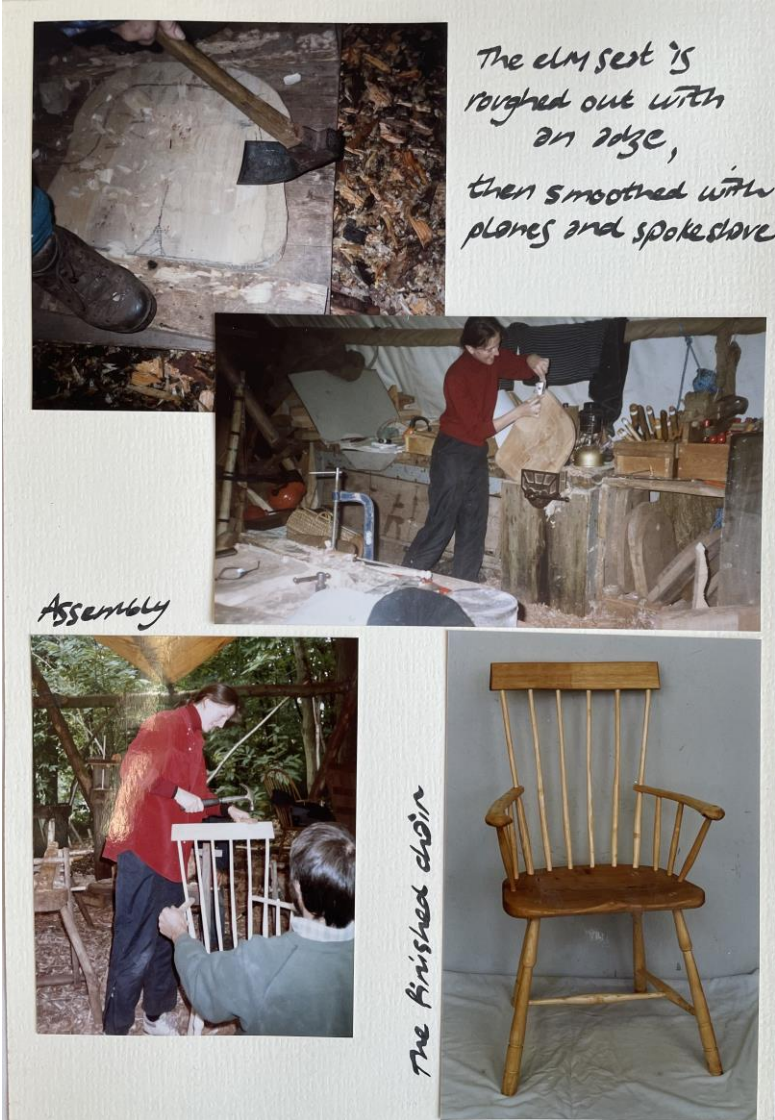
Figures 15-16. Scrapbook pages with photographs from a green woodworking course I took with Mike Abbott in Somerset, 1994. Showing (from top left) felling the tree, working on the shaving horse, steam bending, (from top right) roughing out the seat with an adze, shaping the seat with a spokeshave, assembling the chair with Mike, the finished chair. Photographer unknown.
