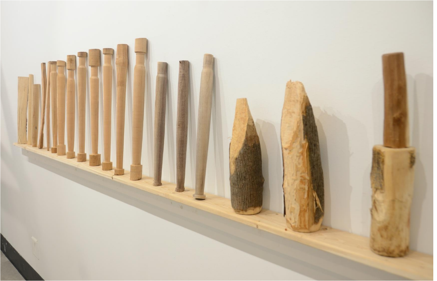
Figure A4. Ledge 1 showing split sections of logs, experiments in turning tapered cylinders for stool legs, gluts and a mallet. Ash, cherry, walnut, mulberry. 2022-2024.
