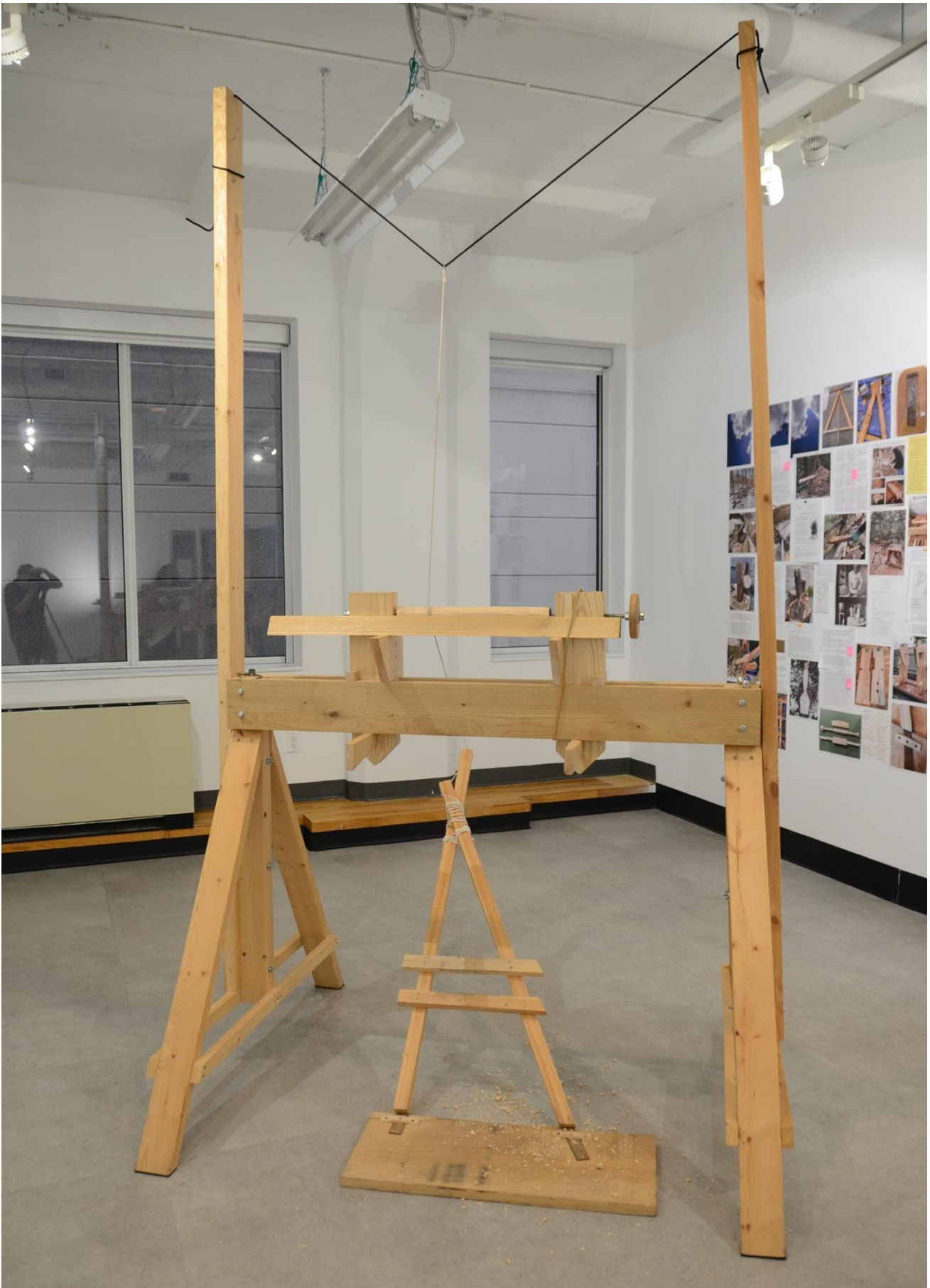
Figure A6. Pole lathe. Oak, ash and SPF, bungy cord, nylon cord, leather. August 2022.
