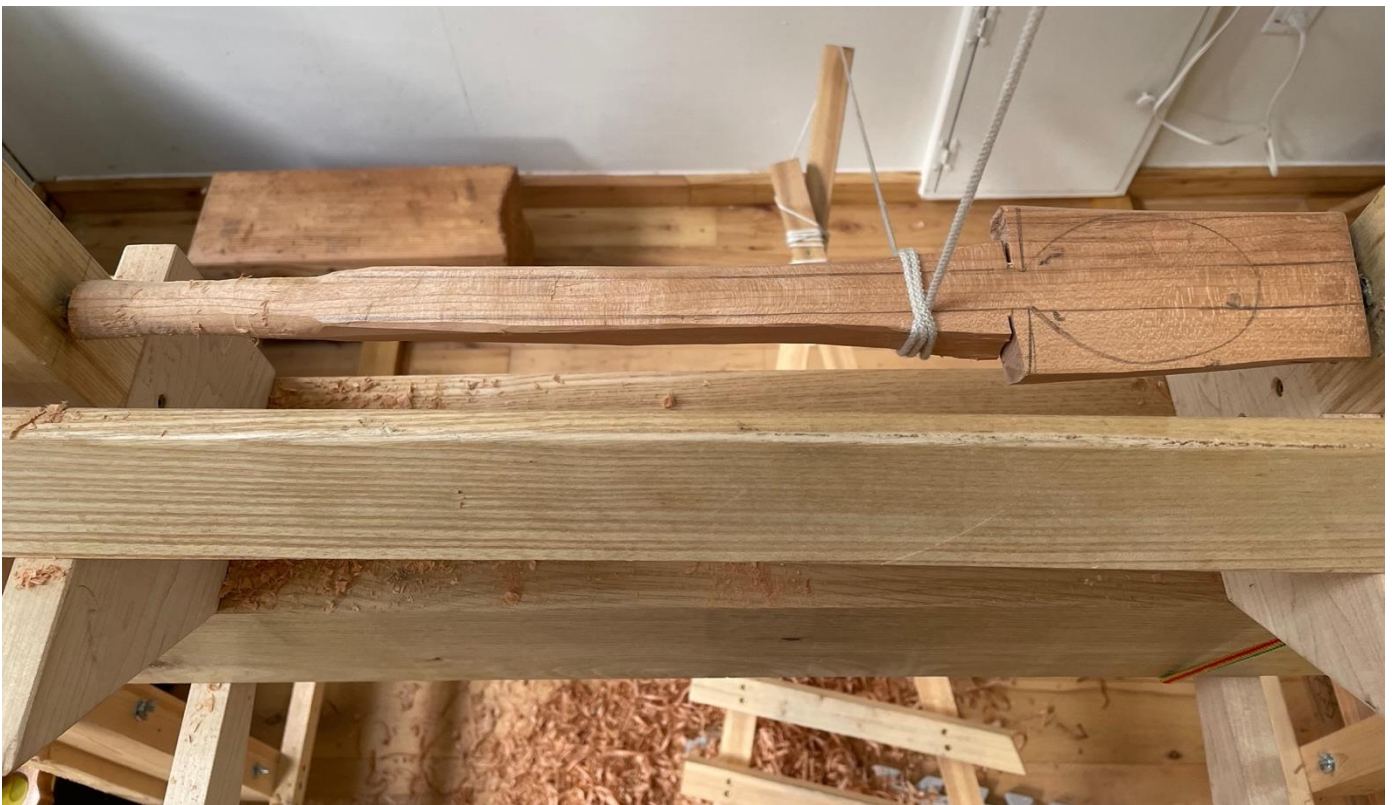
Figures 21-22. Ongoing experiments in spoon carving. Top: Shown in order of making; first attempt on the far left. The neck was too narrow and eventually snapped. Maple, alder, walnut. Bottom: Turning a long-handled spoon on the pole lathe. Cherry. 2022-4.
