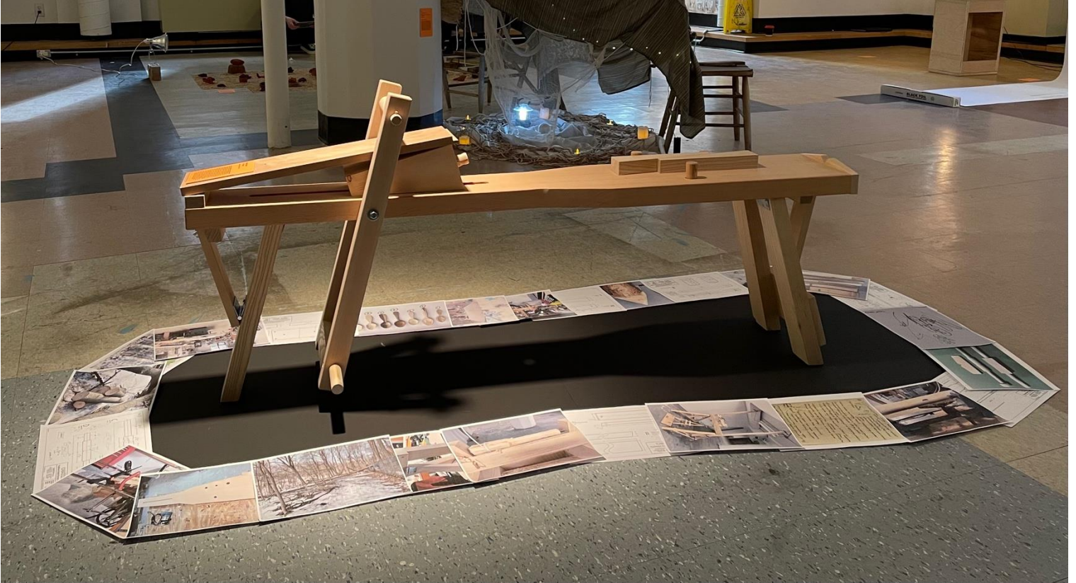
Figure 3. Shaving horse shown here in a class exhibition at OCAD University. Douglas fir, maple, ash, cherry. On the ground: photographs, notes, schematics and cutting lists from the making process. April 15, 2022.
