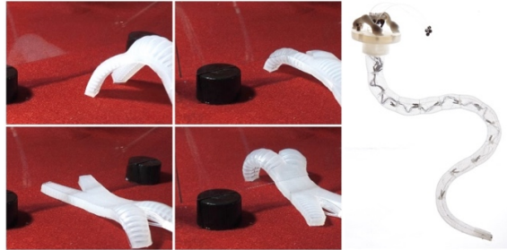
Figure 107 - Left image: 'Multigait soft robot' by (Shepherd et al., 2011) - right image: 'Flexible octopus-like robot arm', photographed by Massimo Brega
