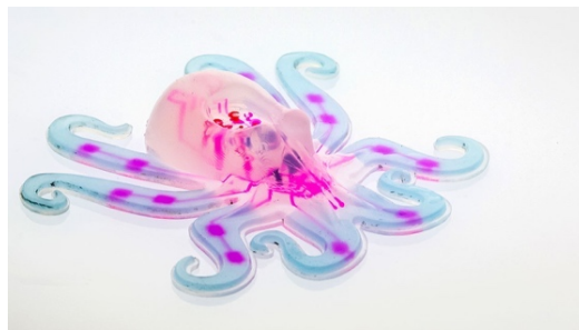
Figure 108 - Octobot, soft autonomous robot by Harvard University (Wehner et al., 2016)
