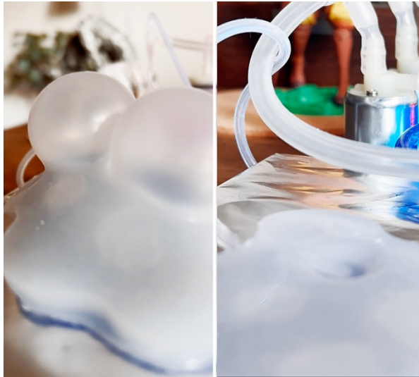
Figure 40 - Prototype I, inflate and deflate states - fabricated and photographed by author
