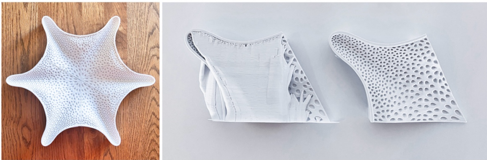
Figure 87 - Symbiont's Mold - Top Part, Right Image: single part before and after removing 3D print's supports, designed and fabricated by author
