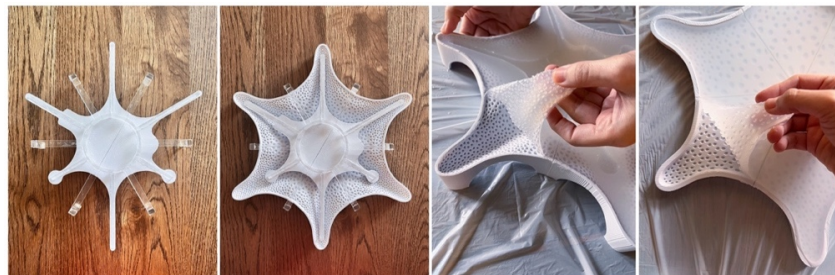
Figure 90 - Symbiont's Mold - Creating Cavity using Bone Structure and Casting the Body, designed and fabricated by author
