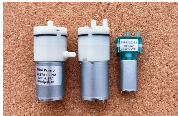
Figure 49 - Air Pumps Tested in Prototype II, version II, photographed by author
