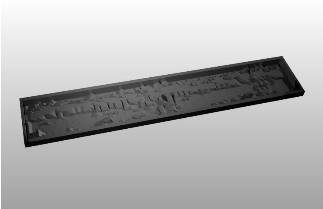
Figure 7.11. Rhino export of the 3d Mesh that was sent to the Rapid Prototyping Center for CNC Milling.
